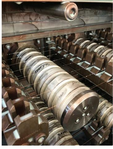
maintenance, we keep Izory®HD drawing rings and rolls in stock for a number of standard machines including those made by Niehoff, MFL, SAMP, Syncro and Henrich.
