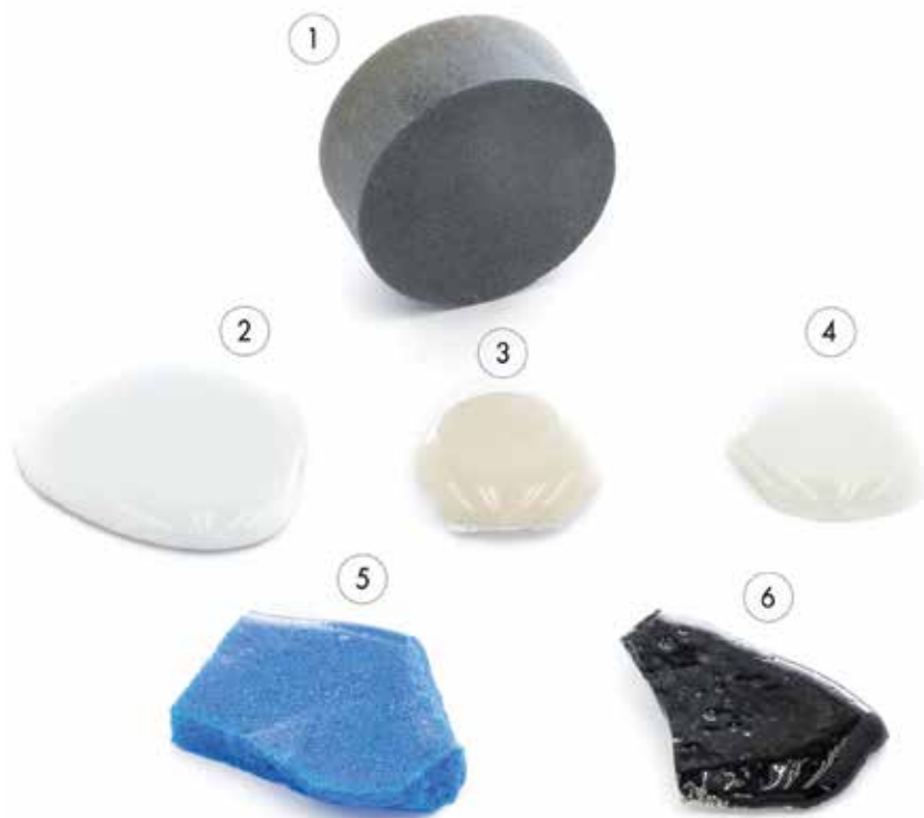
Figure 2. Examples of non-machined materials used for experiments: (1) porous alumina grit puck bonded with glass (no boron); (2) borosilicate glass produced from frit powder; (3) glass, no boron; (4) borosilicate glass; (5) vesicular borosilicate glass with Cu^{2+} ; and (6) borosilicate glass with Cu^+ and roughened surface.
